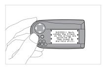
Next orient the G-tech as shown with the arrows pointing up, and press ...
