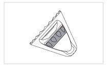
Insert the suction cup into the mounting bracket.
