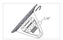
Place the Small Tensioning Nut on the threaded spindle, and turn it clockwise a until it is snug on the stem. There should be a small gap between the Small Tensioning Nut and the Large Vacuum Nut.
