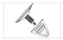
Turn the suction cup clockwise into the Large Vacuum Nut until approximately 1/4 inch of threads protrude.
