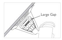
Push the Large Vacuum Nut firmly towards the windshield to expel all air between the suction cup and the windshield. **This is a very important step to ensure proper operation of the mounting system**.
