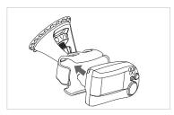
Plug the large end of the DC power cord into your vehicle's 12V cigarette lighter socket. The G-tech will power on.
